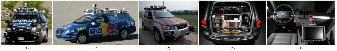
Figure 3: DARPA Urban Challenge (a) CMU's Boss (b) Stanford's Junior (c) Virginia Tech's Odin (d) Computing system (e) Drive-by-wire system and the interface for manual vehicle operation [12]
