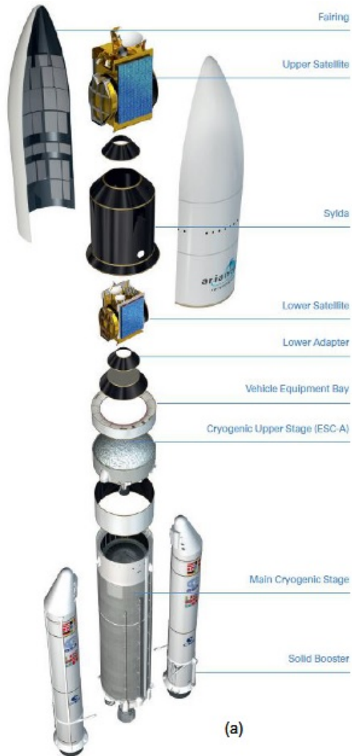
Figure 6: Ariane-5 launch vehicle and the launch infrastructure at the Guiana Space Center (CSG) [1]
